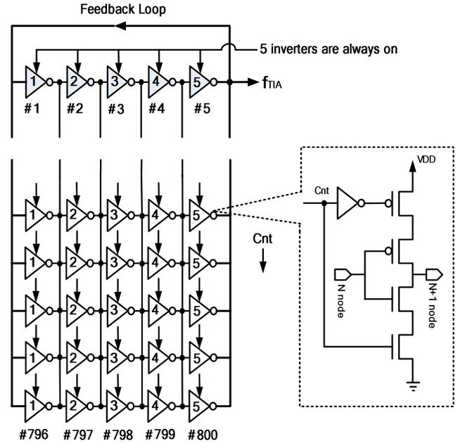
Figure 2. The schematic of tri-state inverter array
