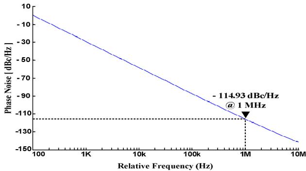
Figure 11. Simulated phase noise for 5A channel frequency
