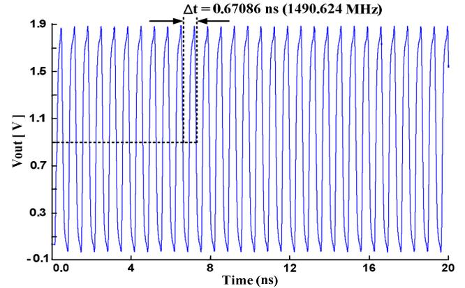
Figure 10. Simulation result of LW channel frequency synthesis
