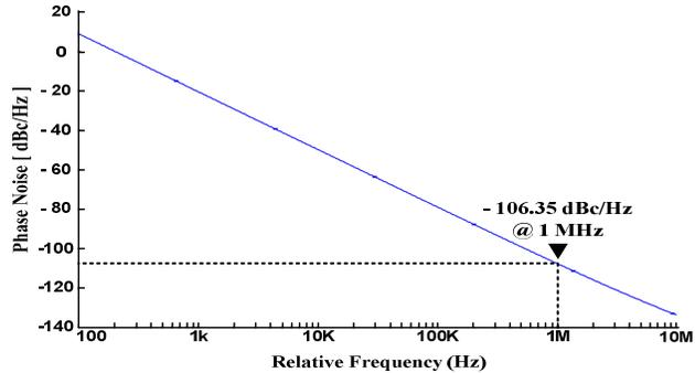
Figure 12. Simulated phase noise for LW channel frequency
