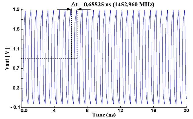
Figure 9. Simulation result of LA channel frequency synthesis
