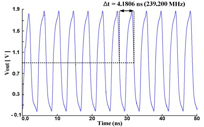
Figure 8. Simulation result of 13F channel frequency synthesis
