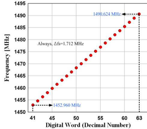
Figure 5. L-BAND frequency versus digital word
