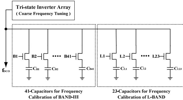
Figure 3. Frequency calibration block for fine tuning
