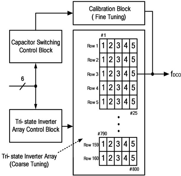
Figure 1. Block diagram of the DCO
