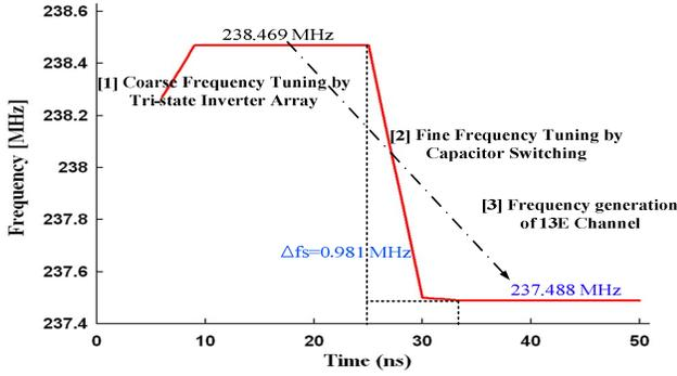
Figure 6. Frequency generation procedure of 13E channel
