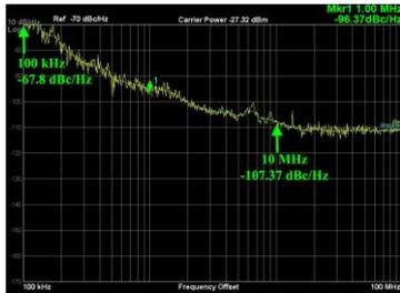
Fig. 1. Measured phase noise of META-VCO
