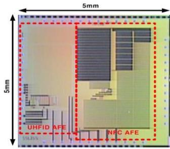
Figure 4. Photograph of the dual-band smart-tag chip
