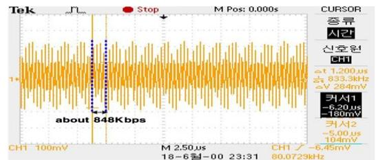
Figure 9. The signal after sending the response signal
