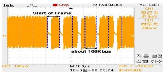
Figure 6. Measurement of the reader signal
