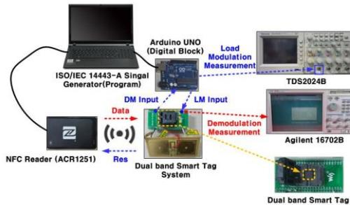
Figure 5. Measurement Environment
