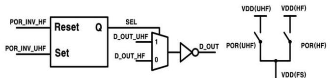
Figure 3. The proposed frequency selector circuit
