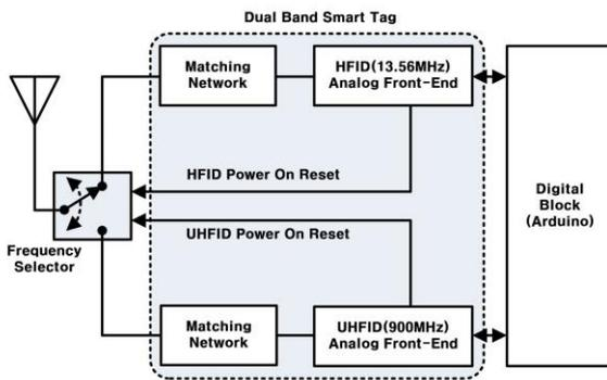
Figure 1. Block diagram of the proposed dual-band smart tag
