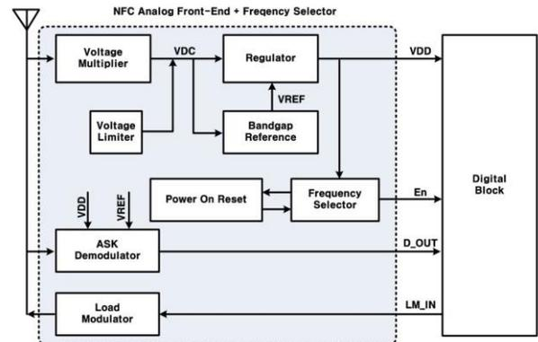
Figure 2. Block diagram of the proposed analog front-end
