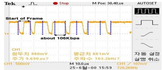
Figure 7. Measurement of the demodulation signal
