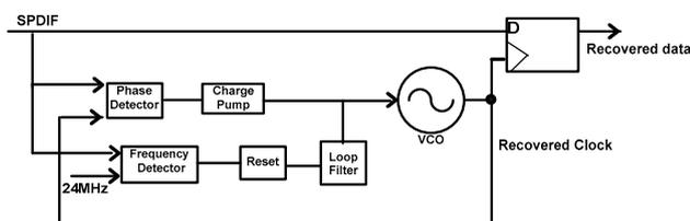
Figure 1. PLL-based CDR Block Diagram
