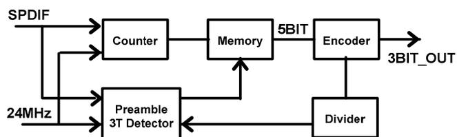
Figure 2. Frequency Detector Block Diagram
