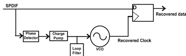
Figure 3. The CDR based on PLL Block Diagram
