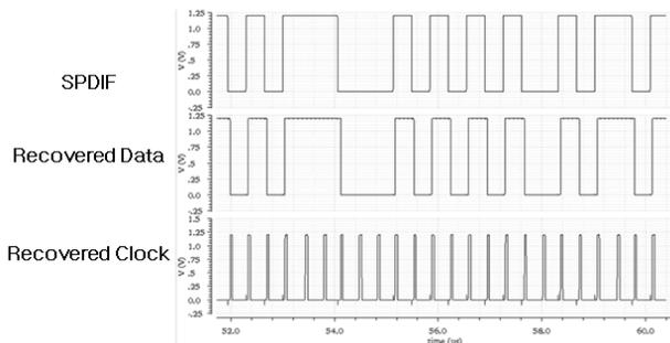
Figure 7. SPDIF/ Recovered clock / Recovered data Graph
