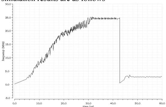
Figure 6. Recovered clock Frequency
