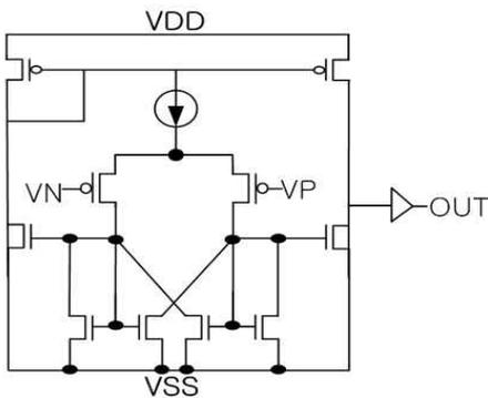
Fig. 4 Hysteresis comparator circuit
