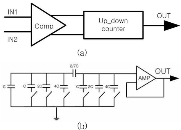
Fig. 6 (a) 6bit ADC and (b) 6bit DAC circuit
