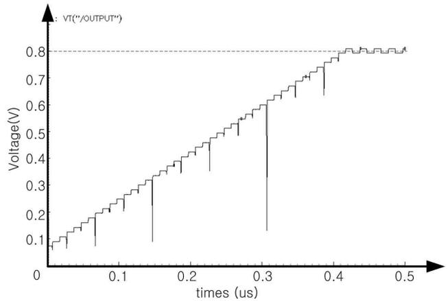
Fig. 9 The output of ADC-DAC loop
