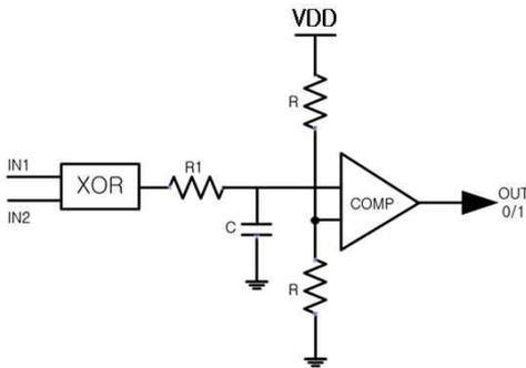
Fig. 3 Lock Detection Circuit
