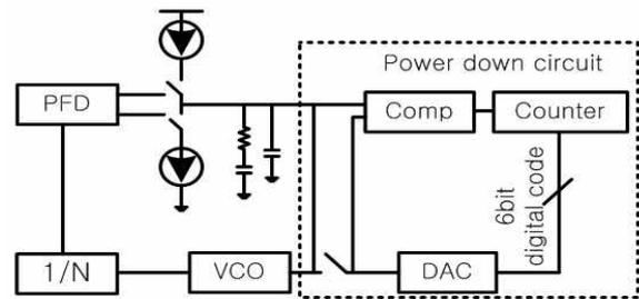
Fig. 5 Proposed PLL with Power Down circuit
