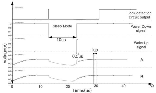
Fig. 10 The locking states of the proposed PLL(A) and the conventional PLL(B).
