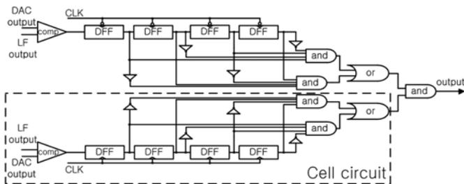
Fig. 3 Lock detection circuit
