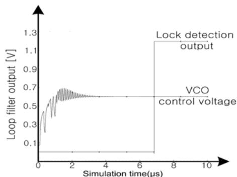
Fig. 8 The locked state of PLL
