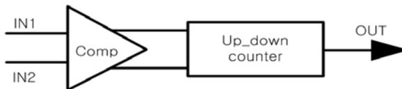
Fig. 5 7 bit ADC circuit
