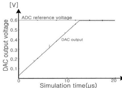
Fig. 7 The output of ADC-DAC loop
