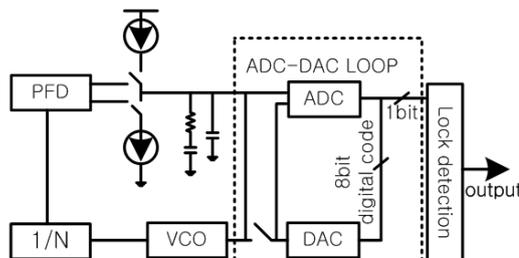
Fig. 2 Block diagram of lock detection
