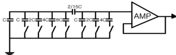
Fig. 4 7 bit DAC circuit
