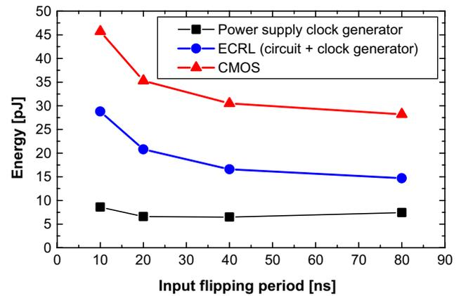
Fig. 11. The energy consumption of a 16×8-bit shift register file when ‘enable’ signal is always on.
