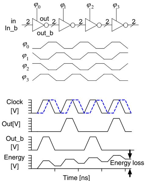
Fig. 2. The energy recovery of an ECRL inverter chain.
