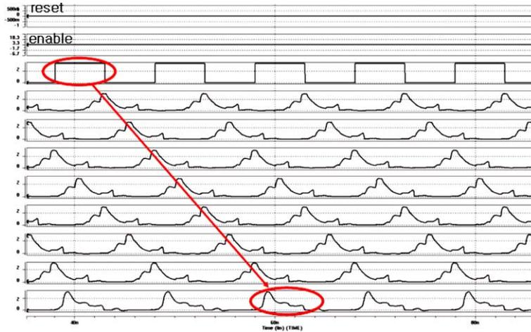
Fig. 9. The SPICE simulation result of a 16×8-bit shift register file.
