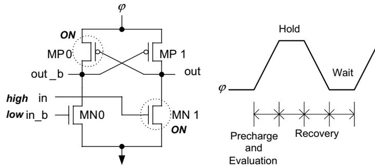
Fig. 1. The basic structure of an ECRL inverter and operation phases of supply clocks.
