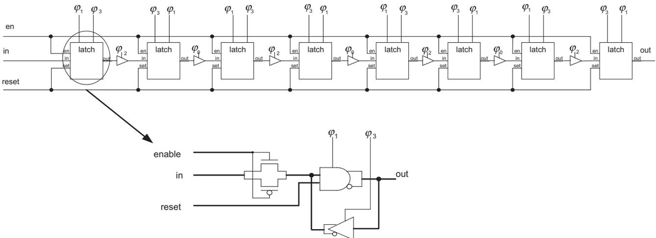
Fig. 8. The structure of a  $16 \times 8$ -bit shift register file.
