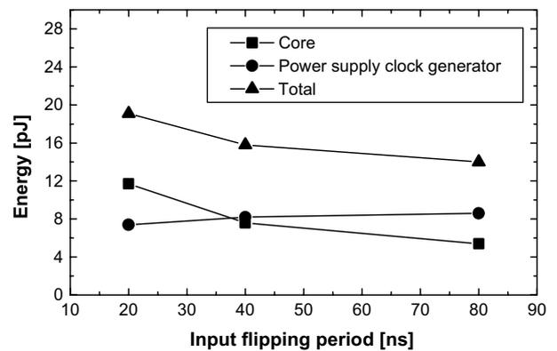
Fig. 12. The energy consumption of a 16×8-bit shift register file for the case that ‘enable’ signal is ‘1’ only when input values are changed.
