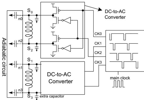
Fig. 7. The schematic of the power supply clock generator.
