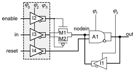
Fig. 3. The schematic of an ECRL latch.
