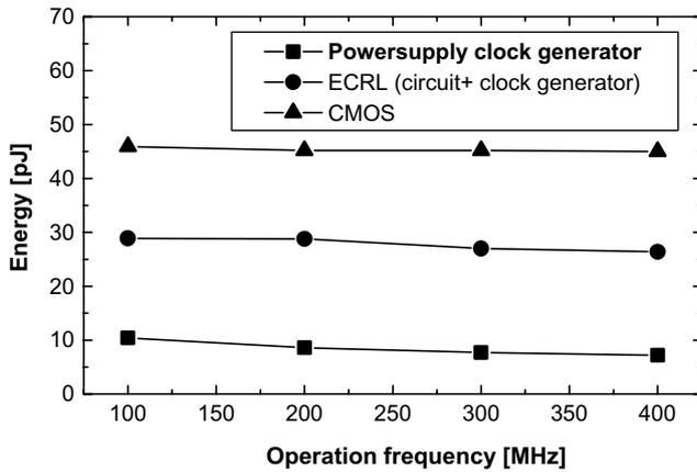
Fig. 10. The energy consumption of a 16×8-bit shift register file for the various supply clock frequencies.
