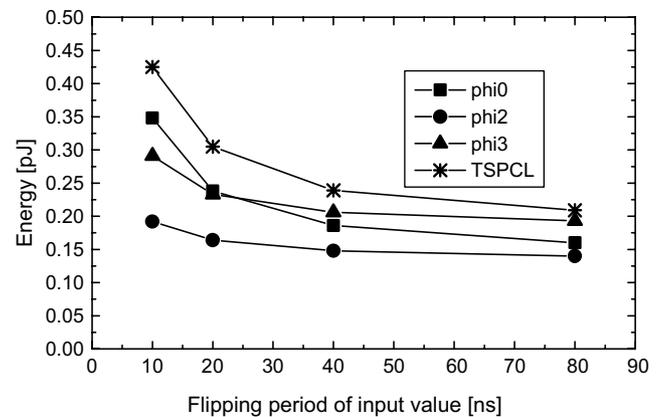
Fig. 5. The energy consumption of the ECRL latch and the CMOS TSPCL FF when ‘enable’ signal is always on.
