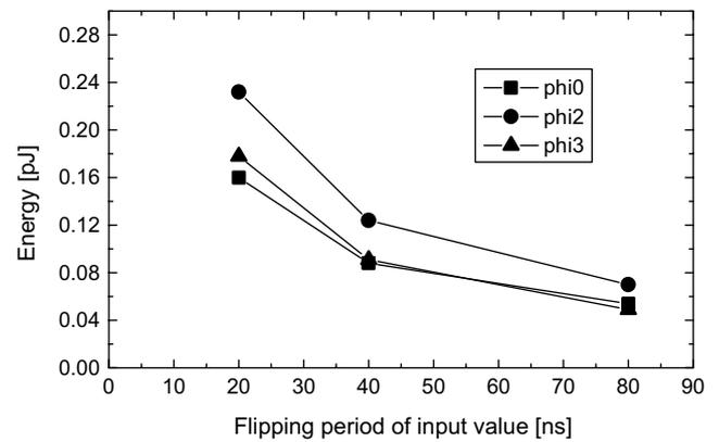
Fig. 6. The energy consumption of the ECRL latch for the case that ‘enable’ signal is ‘1’ only when input values are changed.
