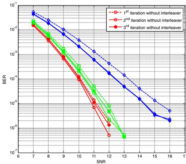
**Fig. 5.** (Color online) BER performance without an interleaver. The curves of the circle, square, and diamond markers represent the performance of no misalignment, (10%, 10%) misalignment, and (20%, 20%) misalignment, respectively.
