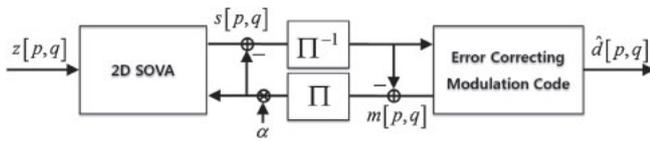
Fig. 1. Turbo equalizer with 2D SOVA and error-correcting modulation code.
