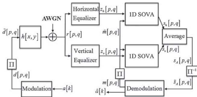
Fig. 2. Block diagram of the whole system.
