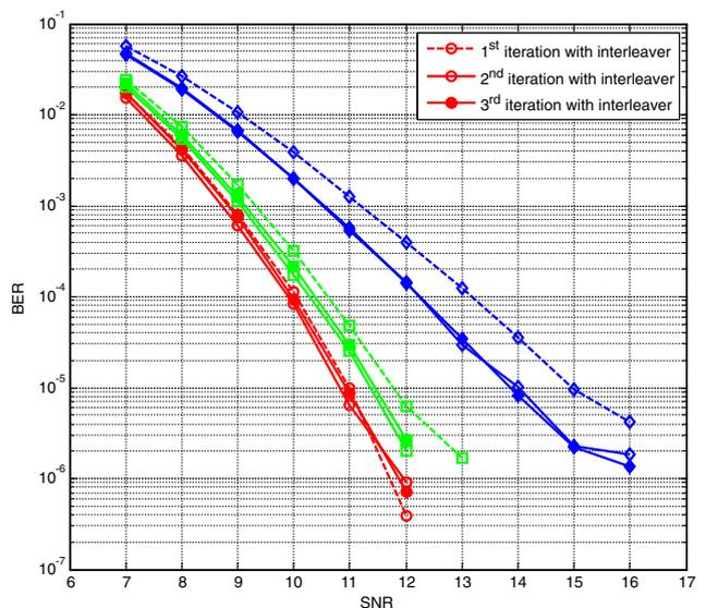
Fig. 4. (Color online) BER performance with an interleaver. The curves of the circle, square, and diamond markers represent the performance of no misalignment, (10%, 10%) misalignment, and (20%, 20%) misalignment, respectively.
