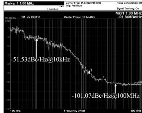
Fig. 14. Measured phase noise versus offset frequency
